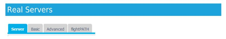
The **Server** tab contains the **Real Server** details associated with the highlighted **Virtual Service**. You will be prompted to add at least one **Real Server** when setting up a **Virtual Service**.
